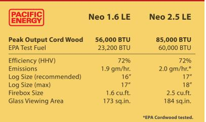
The Neo 1.6 LE makes a bold statement with it's tall profile for easy loading, line-of-sight view of the flame, and modern design. Like its larger cousin the Neo 2.5 LE, the Neo 1.6 LE is a true heating machine with Pacific Energy's solid steel construction and floating firebox with stainless steel baffle. Choose the color that is right for your home with side panels available in a variety of porcelain enamel colors.
