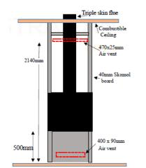
CLEARANCES BASED ON INSTALLATION HAWKWIND 200MM TRIPLE SKIN FLUE KIT. UNIT TO BE PLACED ON A BOX 1000MM[w] x 400MM[h] x 470MM[d] MADE FROM 50MM SKAMOL
